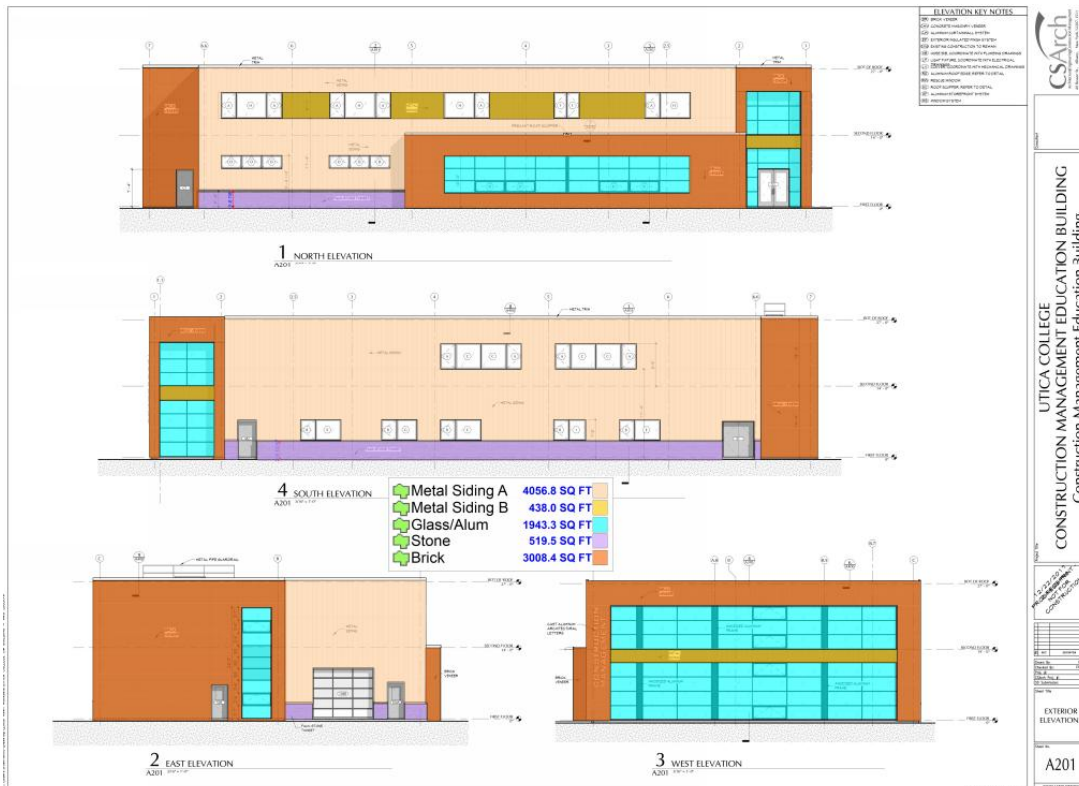
Figure 1. Exterior Elevations Contractor’s Takeoff in PlanSwift
