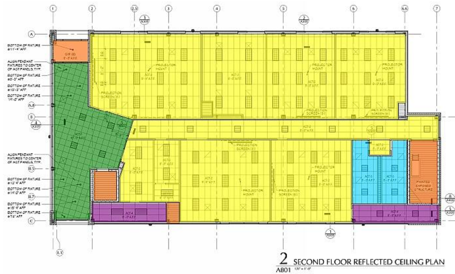
Figure 3. Reflected Ceiling Plan Takeoff Contractor
